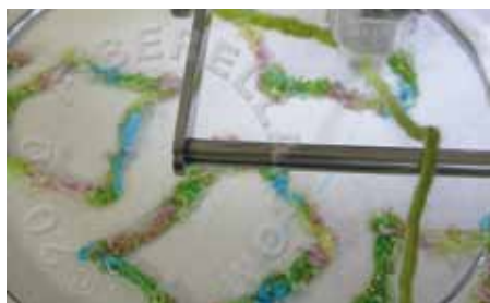
Medium yarn enters back of foot. Large and fine materials enter front of foot.
